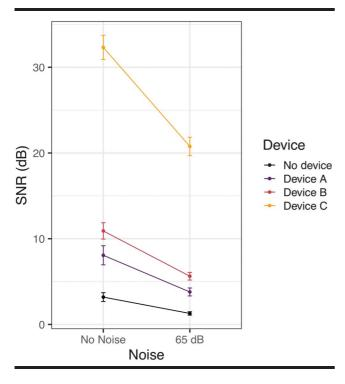
followed by Device B (NN: 10.91 dB; noise: 5.63 dB), and then Device A (NN: 8.07 dB; noise: 3.79 dB).
